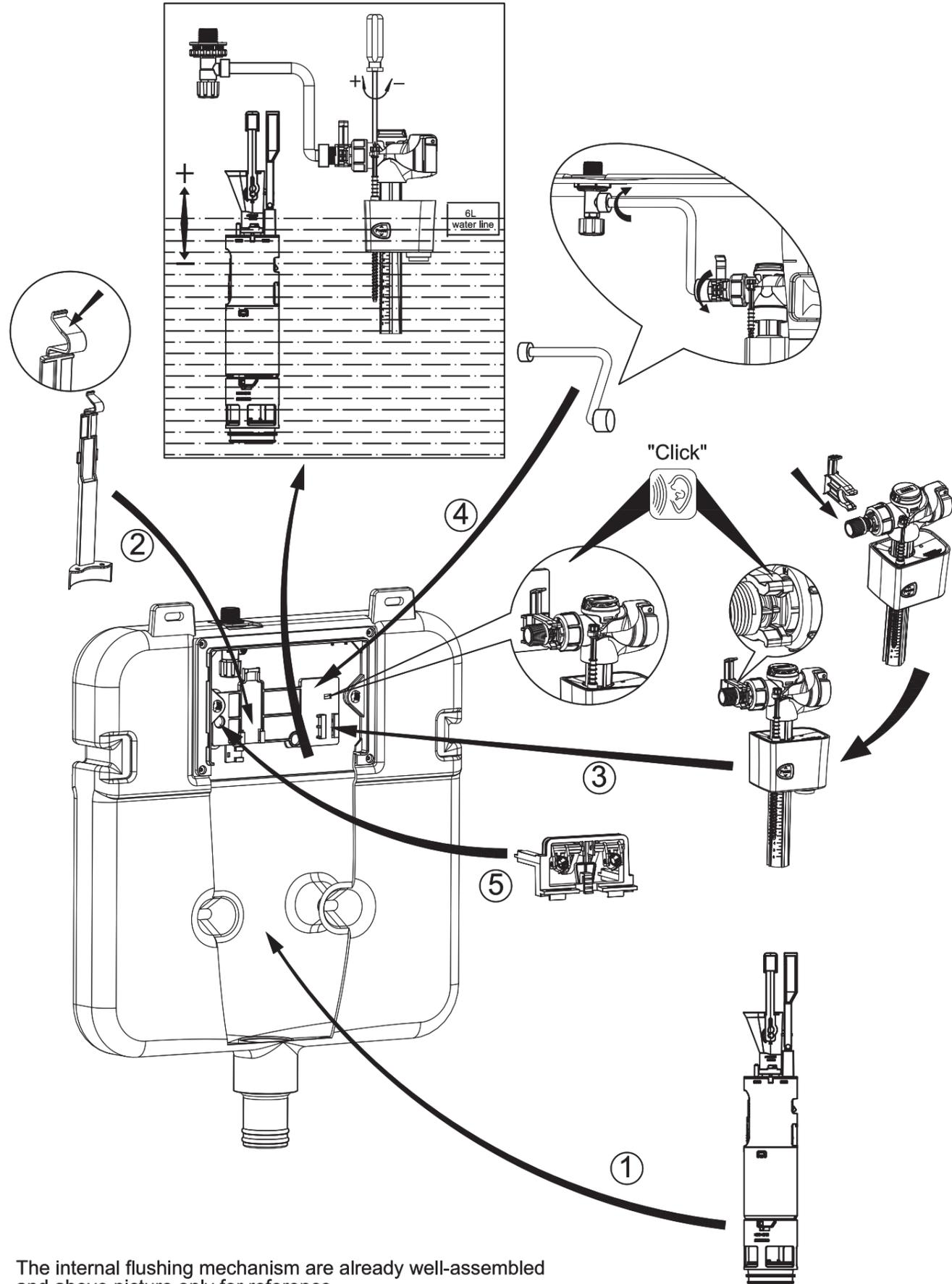
The internal flushing mechanism are already well-assembled and above picture only for reference.
